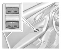
The power windows work when the vehicle is on, in accessory mode, or when Retained Accessory Power (RAP) is active. See *Retained Accessory Power (RAP)* ⇒ 195.
