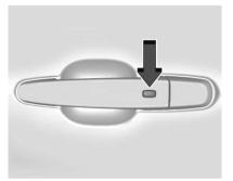
The remote key must be within 1 m (3 ft) of the liftgate or door being opened. Press the button on the door handle to unlock. See "Keyless Access Operation" in *Remote Key Operation* ⇔ 7.
