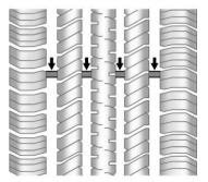
Treadwear indicators are one way to tell when it is time for new tires. Treadwear indicators appear when the tires have only 1.6 mm (1/16 in) or less of tread remaining. See *Tire Inspection*  $\Leftrightarrow$  293 and *Tire Rotation*  $\Leftrightarrow$  293.
