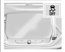
To turn off only the Traction Control System, press and release  $\frac{1}{24}$ . The Traction Off light  $\frac{1}{24}$  displays in the instrument cluster and a Driver Information Center message may display.
