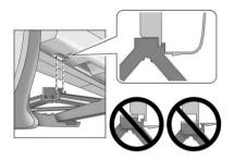
5. Turn the wheel wrench clockwise to raise the jack until the slot in the jack lift head fits into the metal flange located behind the cut out on the plastic molding.
