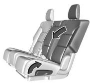
2. Pull the handle on the side of the seat cushion to unlock it.
