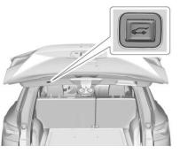
Press any liftgate button or the touch pad while the liftgate is moving to stop it. Pressing again restarts the operation in the reverse direction. The touch pad in the liftgate handle cannot be used to close the liftgate.
