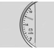
When the ignition is on, this gauge indicates the battery voltage.
