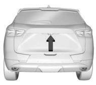
Dirt, snow, or other debris blocks the camera lens. Clean the lens with a soft damp cloth, or if equipped, with the Rear Camera Washer. See *Rear Window Wiper/Washer* ⇒ 89. • The camera's mounting on the vehicle has been damaged, and/or the position or the mounting angle of the camera has changed.
