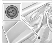
If equipped with a power liftgate, the switch is on the driver door. The vehicle must be in P (Park).
