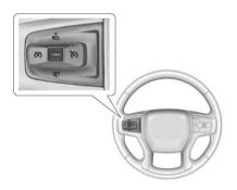
$\mathfrak{S}$ : Press to turn cruise control on or off. A white indicator light is displayed in the instrument cluster when cruise control is turned on.
