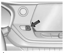
A: Press this button to make the front and rear turn signal lamps flash on and off. This warns others that you are having trouble. Press again to turn the flashers off.
