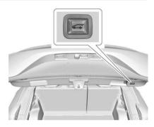
• Press c on the bottom of the liftgate next to the pull cup to close.
