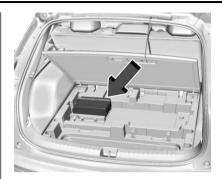
3. Release the strap securing the tire sealant and compressor kit, then remove the kit.
