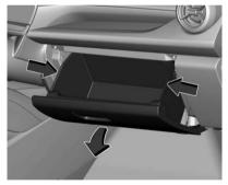
1. Open the glove box door completely.
