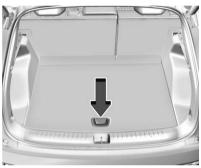
There is storage under the load floor. Press the handle, pull up the load floor, and secure with sky hook to access.
