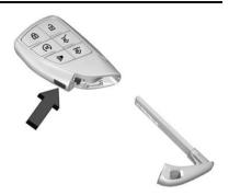
Press the button on the side of the remote key near the bottom and pull the mechanical key out. Never pull the mechanical key out without pressing the button.
