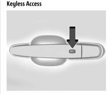
The remote key must be within 1 m (3 ft) of the liftgate or door being opened. Press the button on the door handle to unlock. See "Keyless Access Operation" in *Remote Key Operation*  $rac{1}{2}$  7.
