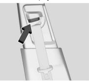
Press the release button and move the height adjuster to the desired position. The adjuster can be moved up by pushing the slide/trim up. After the adjuster is set to the desired position, try to move it down without pressing the release button to make sure it has locked into position.
