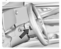
Regen on Demand allows for increased deceleration by pressing and holding the steering wheel paddle. Regen on Demand works in D (Drive). The accelerator pedal can be used to manage deceleration while using Regen on Demand. See One-Pedal Driving \$ 173.
