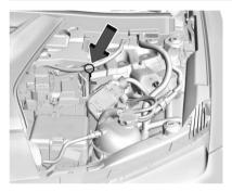
2. Pull the emergency manual charge cord release handle. The DC charge cord will release.
