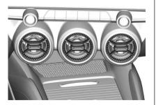
Use the air outlets in the center and on the side of the instrument panel to direct the airflow. Turn the center knobs on the air outlets counterclockwise or clockwise to open or close off the airflow.
