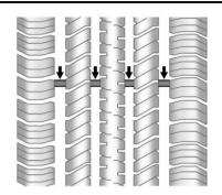
Treadwear indicators are one way to tell when it is time for new tires. Treadwear indicators appear when the tires have only 1.6 mm (1/16 in) or less of tread remaining. See *Tire Inspection*  $\Rightarrow$  299 and *Tire Rotation*  $\Rightarrow$  300.
