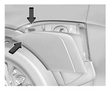
2. Push the top left corner of the charge port door and release to open the door.
