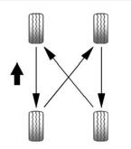
Use this rotation pattern if the vehicle is equipped with front wheel drive.
