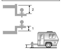
It is important to level the trailer front to back by selecting the correct trailer hitch draw-bar drop (2) or rise (1). Towing with a trailer that is not level can result in incorrect loading of trailer axles, springs, and tires. A trailer that is not level increases the risk of damaging your trailer, trailer sway, and trailer tire blowouts.
