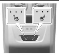
If equipped, the buttons are on the rear of the center console.
