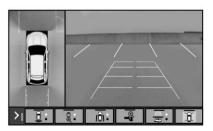
Touch the camera view buttons on the infotainment display to access each view, if equipped. Some views may automatically display, or switch based on vehicle movement or additional safety features. For views that use a shared button, the button to activate the view may be pressed multiple times to switch between them:
