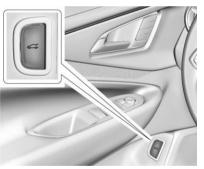
Press c on the driver door. The driver door must either be unlocked or locked without the security armed.
