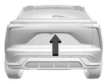
To open the liftgate, press and on the power door lock switch or press and on the remote key twice to unlock all doors. Press the touchpad on the underside of the liftgate handle and lift up.
