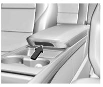
Press the button to access the storage in the center console.
