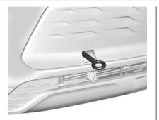
2. Install the tow eye into the socket and turn it until it is fully tightened. When the tow eye is removed, reinstall the cover with the notch in the original position.
