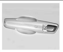
2. Insert the cap back into the grooves on the door handle.
