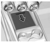
To open the front storage compartment, slide the cover forward. There are two USB ports inside. To close, push the cover forward and let go.
