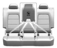
Do not install a child restraint that requires lower anchors in the center rear seating position. See Securing Child Restraints (With the Seat Belt in the Rear Seat)  $\Rightarrow$  70 Securing Child Restraints (With the Seat Belt in the Front Seat)  $\Rightarrow$  72.
