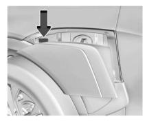
2. Press the button to manually close the charge port door.
