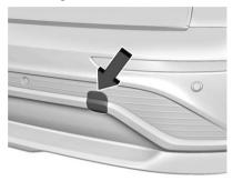
1. Carefully open the cover on the fascia by using the small notch that conceals the tow eye socket.
