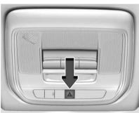
A: Press this button on the overhead console to make the front and rear turn signal lamps flash on and off. This warns others that you are having trouble. Press again to turn the flashers off.
