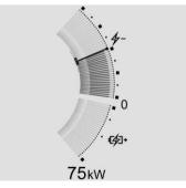
Single Power Indicator Gauge Shown, Others Similar The power indicator gauge is in the center of the display to the right of the speedometer in the Single Gauge layout.
