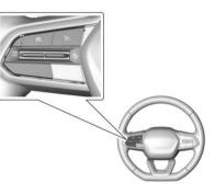
S: Press to turn the system on or off. The ACC indicator light → displays white on the instrument cluster when ACC is turned on.
