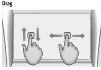
Drag is used to move applications on the infotainment home screen, or to pan the map. To drag the item, it must be held and moved along the display to the new location. This can be done up, down, right, or left. This feature is only available when vehicle is parked and not in motion.
