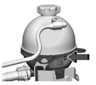
5. If the coolant level is not visible or needs to be adjusted within the reservoir, contact your dealer.
