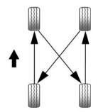
Use this rotation pattern if the vehicle is equipped with rear wheel drive or all wheel drive.
