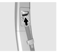
Press and hold the release button while raising or lowering the height adjuster to the desired position.
