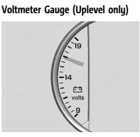
When the ignition is on, this gauge indicates the battery voltage.
