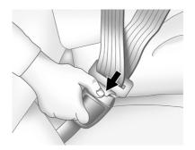
To unlatch the belt, push the release pushbutton on the buckle. The belt should return to its stowed position.
