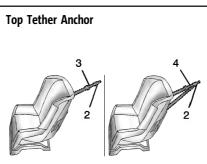
A top tether (3, 4) is used to secure the top of the child restraint to the vehicle. A top tether anchor is built into the vehicle. The top tether attachment hook (2) on the child restraint connects to the top tether anchor in the vehicle in order to reduce the forward movement and rotation of the child restraint during driving or in the event of a crash.
