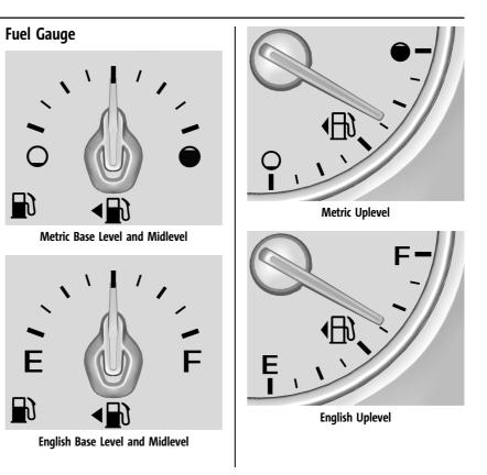
When the ignition is on, the fuel gauge indicates the approximate amount of fuel left in the tank.
