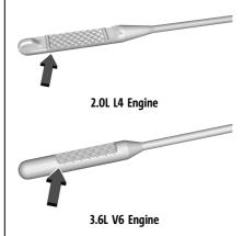
If the oil is below the cross-hatched area at the tip of the dipstick and the engine has been off for at least 15 minutes, add 1 L (1 qt) of the recommended oil and then recheck the level. See "Selecting the Right Engine Oil" later in this section for an explanation of what kind of oil to use. For engine oil crankcase capacity, see *Capacities and Specifications* ⇔ *323*.
