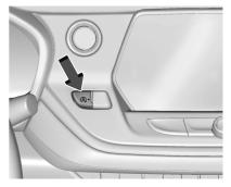
The automatic engine Stop/Start feature can be disabled and enabled by pressing  $\bigcirc$ . Auto Stop/Start is enabled each time you start the vehicle.
