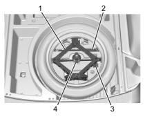
3. Turn the wing nut (4) counterclockwise to remove the jack (1), wheel wrench (2), and strap (3). Place the tool container near the tire being changed.
