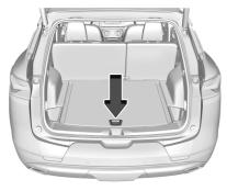
Lift the load floor to access the cargo management system.
