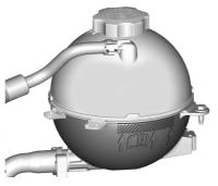
Check to see if coolant is visible in the coolant surge tank. If the coolant inside the coolant surge tank is boiling, do not do anything else until it cools down. See *Engine Overheating*  $\Leftrightarrow$  258.
