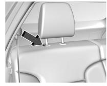
To lower the head restraint, press the button, located on the top of the seatback, and push the head restraint down. Try to move the head restraint after the button is released to make sure that it is locked in place.
