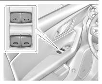
The power windows work when the vehicle is on, in accessory mode, or when Retained Accessory Power (RAP) is active. See Retained Accessory Power (RAP) ⇔ 193.
