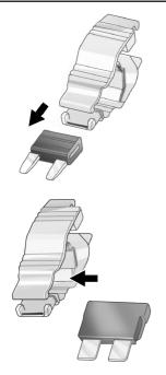
3. Use the fuse puller to remove the fuse from the top or side.
