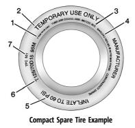
(1) Tire Ply Material : The type of cord and number of plies in the sidewall and under the tread.
