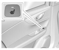
If equipped, the buttons are on the rear doors.
