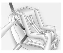
6. To tighten the belt, push down on the child restraint, pull the shoulder portion of the belt to tighten the lap portion of the belt, and feed the shoulder belt back into the retractor.
