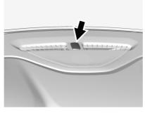
There is a light sensor on top of the instrument panel. Do not cover the sensor.
