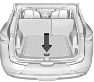
There is storage in the floor of the rear cargo area. Lift the handle to access the cargo management system.
