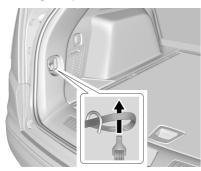
4. Place the loop end of the strap through the cargo tie-down. Place the hook end of the strap through the loop and pull it until the strap is fastened securely to the tie-down.
