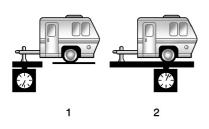
The trailer tongue weight (1) should be 10– 15% of the loaded trailer weight (2). Some specific trailer types, such as boat trailers, fall outside of this range. Always refer to the trailer owner's manual for the recommended trailer tongue weight for each trailer. Never exceed the maximum loads for your vehicle, hitch, and trailer.
