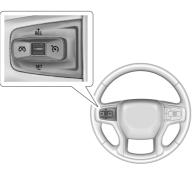
S: Press to turn cruise control on or off. A white indicator light is displayed in the instrument cluster when cruise control is turned on.
